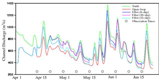
**Figure 3.** Time series of model-predicted discharge at the downstream edge of the channel from different simulations. These include the Truth, Open-loop, and the Filter with 8-, 16-, and 32-day assimilation frequency.
