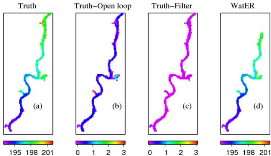
**Figure 1.** Spatial snapshots of WSL (in meters) for (a) the Truth simulation; (b) differences of Open-loop and (c) Filter WSL simulations from the truth; and (d) the satellite observation WSL image assimilated at the timestep shown (28 April 1995, 06:00). The satellite image is an overlay of the left and right viewing angles, with coverage limited by the orbits used in the instrument simulator.
