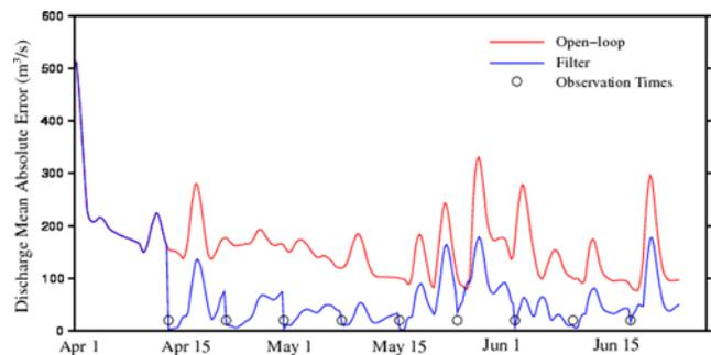
**Figure 2.** Spatially averaged mean absolute error of channel discharge for the Open-loop (red line) and Filter (blue line) simulations. The black circles indicate assimilation times ( $\sim 8$  days).
