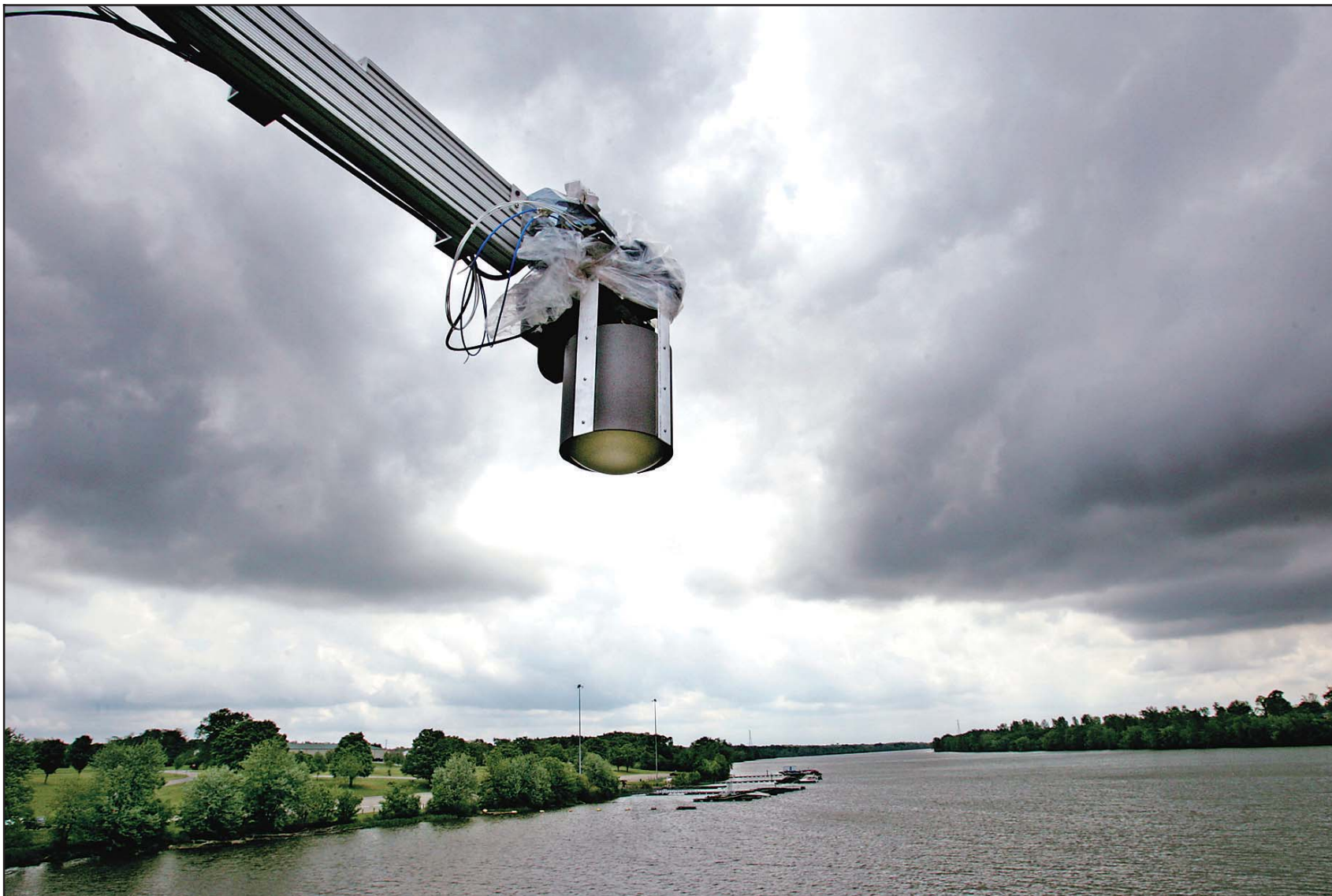
The radar dome hanging over the Scioto River from the Home Road bridge in Delaware County is a prototype, using the KA band, for a future space mission.
