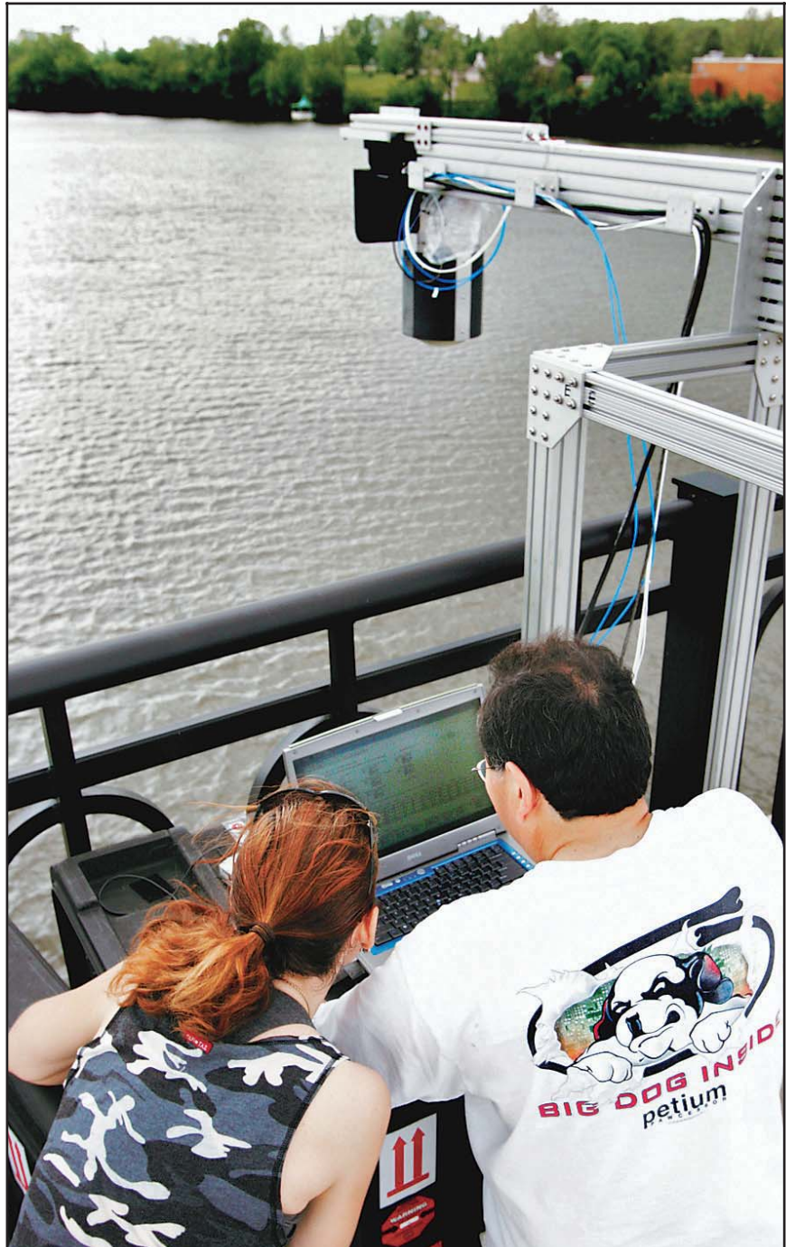
Radar engineers Delwyn Moller, left, and Cliff Yamamoto monitor radar readings on the water at O'Shaughnessy Reservoir on a laptop computer. The research is testing the technology before it is launched into space to monitor all of Earth's water resources.
