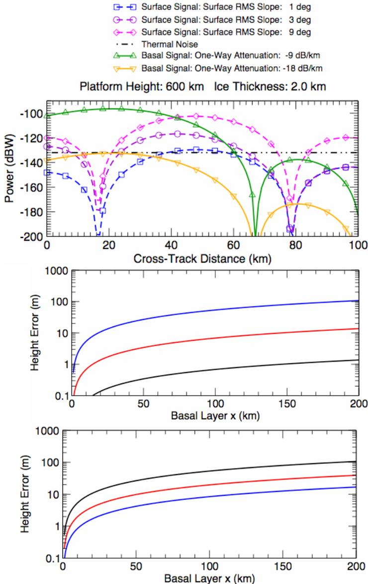
**Figure 1:** Expected signal to noise and signal to clutter ratios for an ice thickness of 2 km and for various surface clutter (which depends on the rms slope of the ice sheet surface) scenarios. As can be seen from this figure, the instrument performance is limited by the clutter.
