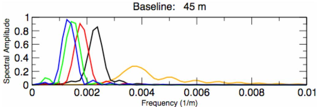
**Figure 3:** *Spectrum of the interferogram for the basal return (orange) and for the surface return for ice depths of 1 km (black), 2 km (red), 3 km (green), and 4 km (blue). The signal to clutter ratio has been assumed to be 0 dB. The spectral amplitude is in relative units. Only positive spatial frequencies are shown.*
