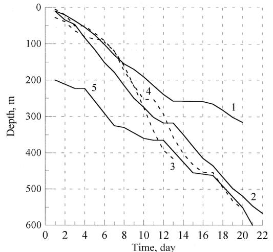
Fig. 7. Progress of boreholes: 1—Windy Dome, m-ATED; 2—Austfonna, ATED; 3—J9, Ross Ice Shelf, ATED; 4—Taylor Dome, PICO electro-mechanical drill; 5—GRIP, electro-mechanical drill.
