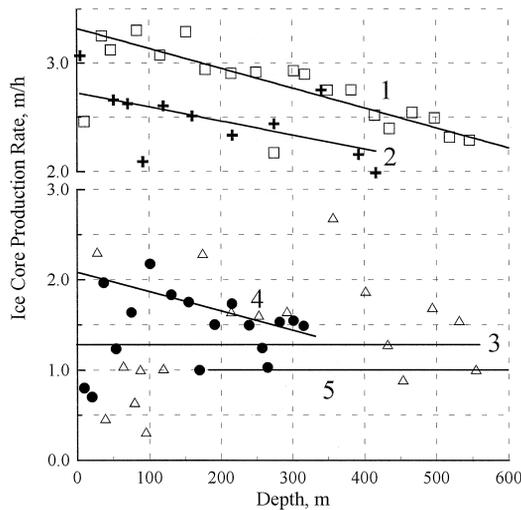
Fig. 1. Mean ice core production rate as function of depth: 1—Austfonna, ATED; 2—J9, ATED; 3—Taylor Dome, PICO electromechanical drill; 4—Windy Dome, m-ATED; 5—GRIP, electromechanical drill.
