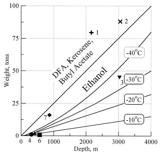
Fig. 8. Borehole liquid requirements: 1—Byrd Station; 2—GRISP2; 3—GRIP; 4—Windy Dome; 5—J9; 6—Austfonna; 7—Komsomolskaya Station; lines are estimation for 180-mm borehole diameter.
