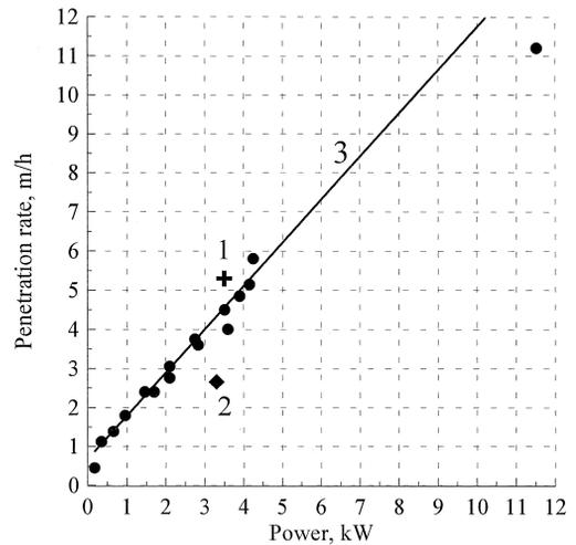
Fig. 3. m-ATED penetration rate as function of power: 1—ATED; 2—m-ATED, EWS circulates through coring head; 3—m-ATED no circulation.
