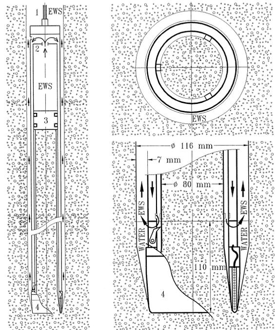
Fig. 2. Schematic of ATED: 1—cable termination; 2—manifold; 3—piston; 4—coring head; arrows show EWS flow.
