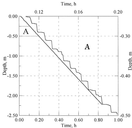
Fig. 6. Depth vs. time during penetration: drilling run #9 in Fig. 5.
