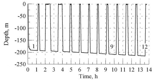
Fig. 5. Windy Dome drilling log data. 11th day of drilling; numbers are drilling runs.
