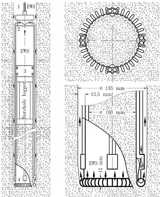
Fig. 4. Schematic of m-ATED: 1—cable termination; 2—memifold; 3—piston; 4—coring head; arrows show EWS flow.
