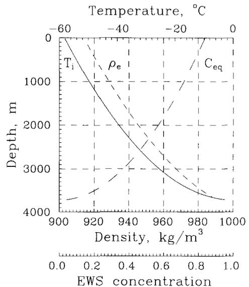
Fig. 4. Calculated temperature of ice ( $T_i$ ), density ( $\rho_e$ ), and concentration ( $C_{eq}$ ) of EWS in the borehole.
