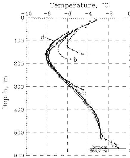
Fig. 5. Temperature distribution in the Austfonna borehole: (a, b, c) measured after break of drilling on respective depth; (d) measured after input of additional ethanol to the borehole.
