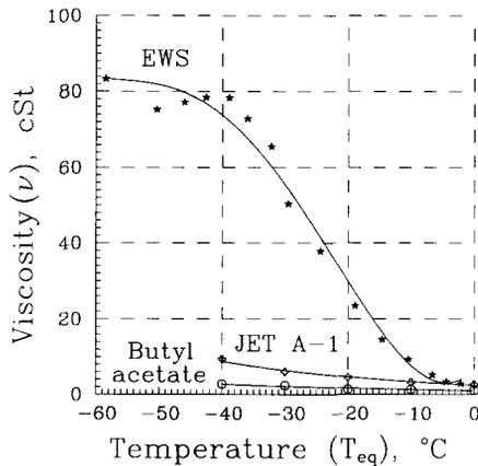
Fig. 3. Viscosity of EWS at equilibrium temperature compared with JET A-1 and butyl acetate.
